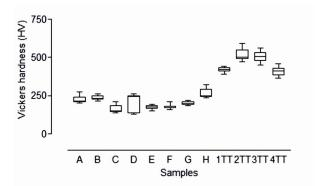
**Figure 2.** Distribution of Vickers hardness values (HV) for 12 distinct samples after mechanical cycling test (A-H) and heat treatment (1TT-4TT). The variance analysis result was significant (P<0.0001). Comparing 2 x 2 by Tuckey test, the results were statistically different (P<0.001) for all samples.
