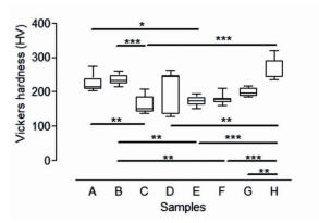
**Figure 1.** Distribution of Vickers hardness values (HV) for 8 distinct samples (A-H) after the mechanical cycling test. The variance analysis result was significant (P<0.0001). Comparing 2 x 2 by Tuckey test, the statistical results can be observed in the figure (\* = P<0.05; \*\* = P<0.01, \*\*\* = P<0.001).
