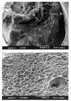
**Figure 3.** SEM images of sample A (a) 50x and (b) 500x regarding the circle, showing the dimples presence, after mechanical cycling test and tensile test.
