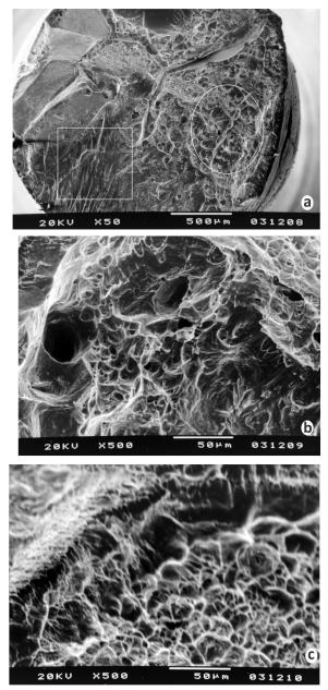
Figure 4. SEM images of sample F (a) 50x and (b) 500x regarding the circle, showing the dimples presence and (c) 500x regarding the square, showing the cleavage presence, after mechanical cycling test.
